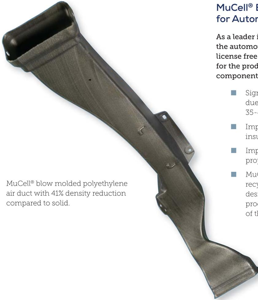
MuCell® blow molded polyethylene air duct with 41% density reduction compared to solid.
